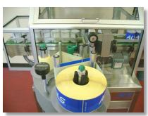
Orientates round products for accurate labelling to a registration mark or weld seam. For full wrap-around or spot labelling applications. Features high accuracy, fast throughput and a heavy-duty, stainless steel construction.
