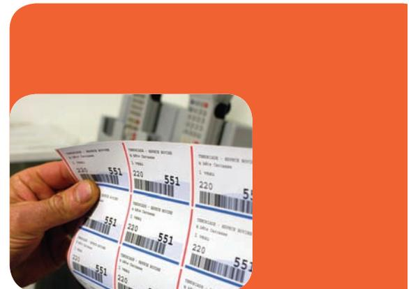
Having checked that the bar codes are in the correct position and are not shortened in height (truncated), you can use verification equipment to obtain an overall grade for each symbol.
