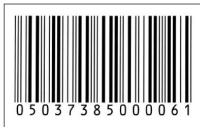
Incorrect adjustment for ink spread (the bar width reduction). The printed bars are out of specification, either being too narrow or too wide.
