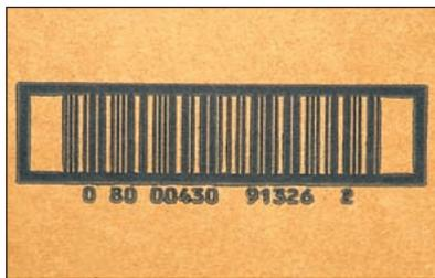
Poor quality substrates are substituted for the original specification, resulting in loss of quality, often greater ink spread, or the appearance of voids in the bars. A darker coloured substrate, for example, could result in insufficient contrast.
