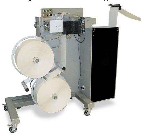
The ASDU features speeds of up to 64 metres per minute and comes equipped with two 500mm unwinds, powered by a high-speed servo drive and is PLC controlled. It is a continuous feed unit designed to roll up to any production line and improve efficiency with minimum operator effort.
