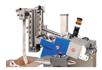
Whizzy Roll is the feeder that cuts and feeds stock on reel on continuous strips, both paper or plastic. The reading of a notch gives a stop signal to the machine, that cuts the products and feeds it. The cut can be performed without the notch reading, by setting the parameters through an optional keyboard.
