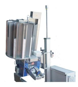
Rotary multistacker feeder for pharma instruction notices with barcode control on dispensing unit. Stackers can be loaded in safety during machine functioning.
