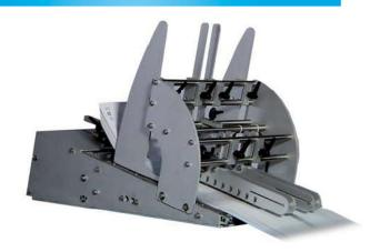
Agile is the new continuous feeder designed by Etipack for most typical applications in mail processing, with folding machines, ink jet bases and labelling bases. Agile is capable of feeding a wide variety of materials, size and weight, at high speed and thus matching the highest output rate perfor-mance with accuracy. Agile is equipped with a special skimming, optional roller for precise product selection and a double belt/double speed system for excellent product distancing (30-40).
