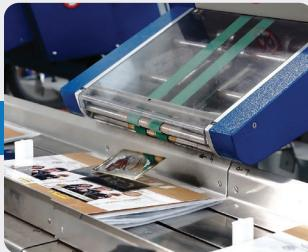
Machines for in-line feeding of products and items such as vouchers, leaflets and others inserts, on-demand. Ideal to integrate with OEM equipment and high-speed precision packaging lines. Suitable for wide variety of applications.
